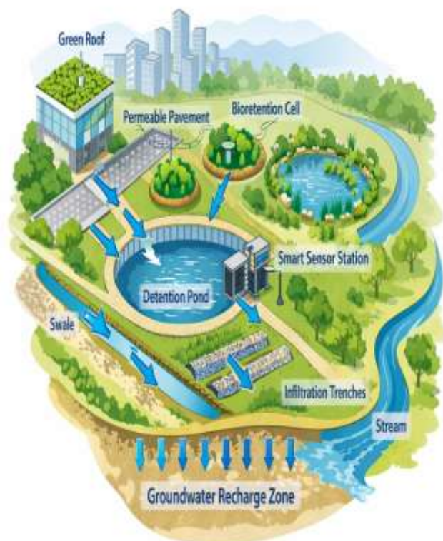
Figure 1. Spatial schematic of SUDS layout integrating drainage and recharge zones (green circles denote bioretention areas; blue arrows show flow paths).
